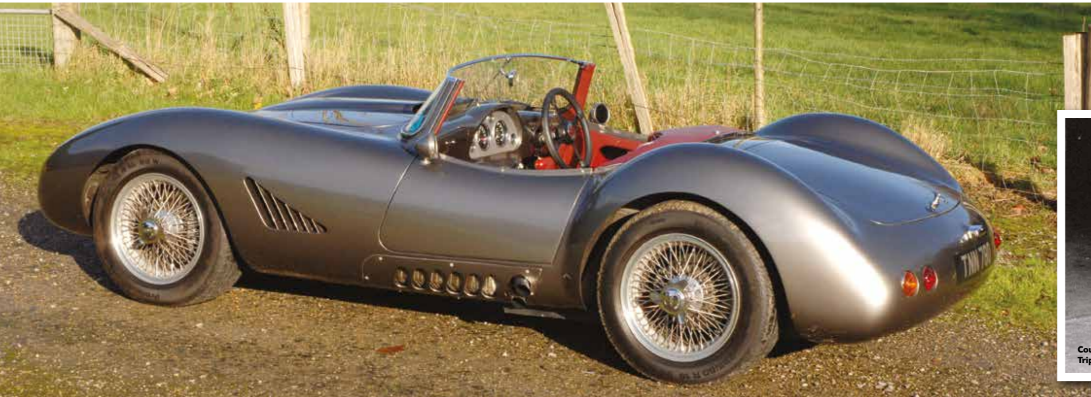
Above: Shades of DBR Aston Martin. Exhaust runs inside the left-hand sill
