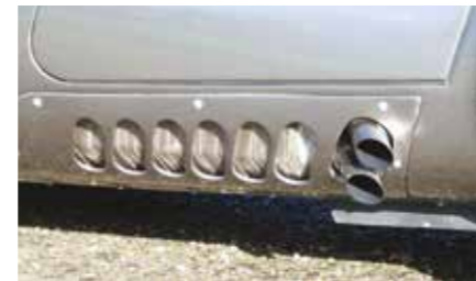
Above: Shades of DBR Aston Martin. Exhaust runs inside the left-hand sill
