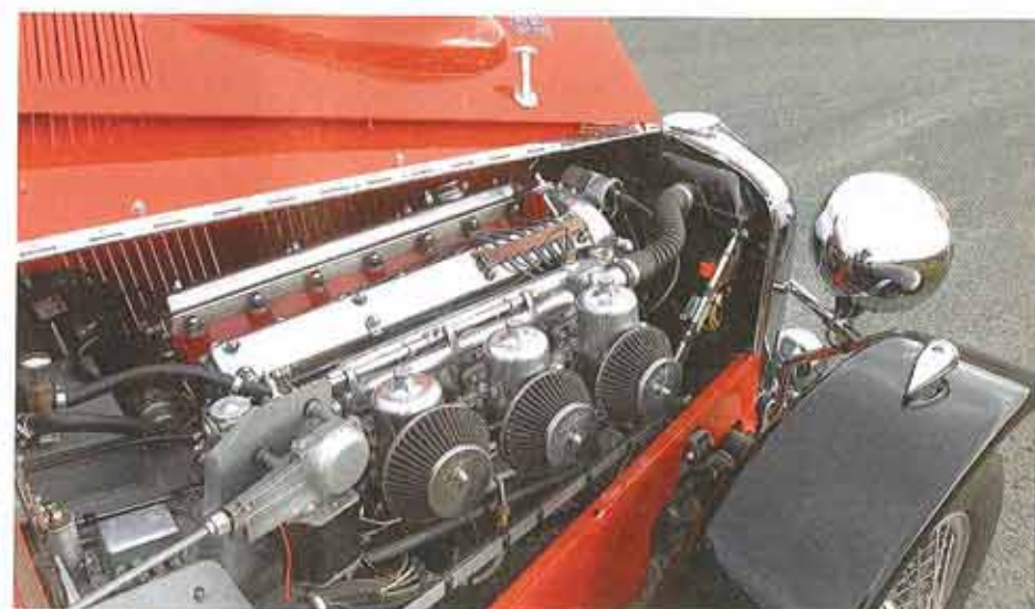
The interior is snug, but comfortable, and is very well thought out – the boot even includes a compartment for a shoe cleaning kit! The 3.4-litre XK engine now features triple carburetors and a straight-port head
