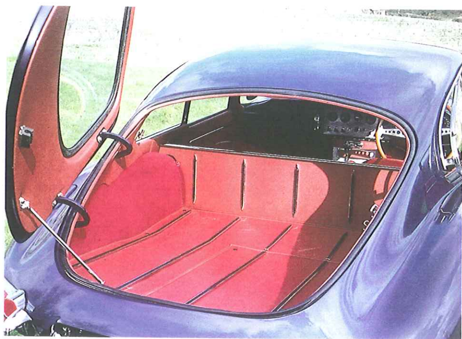
With the fixedhead came an amazing level of practicality. A ribbed load area is perfect for that grand tour with a couple of suitcases on board, and a flip-up end board helps keep the luggage in the rear. A lift-out section (just visible, bottom right) gives access to the spare wheel
