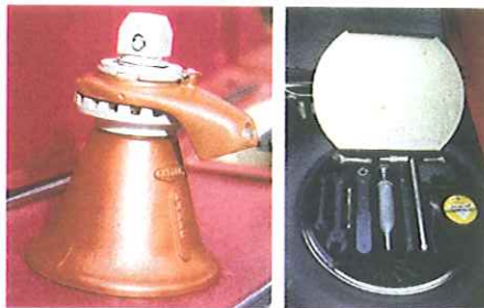
Early cars used a screw-type jack and a Mk 2-style tool kit. Later cars featured a more conventional roll-up kit
